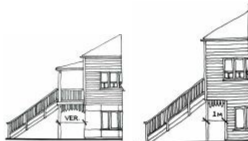
Figure 6.74 - Appropriate enclosures to the ground floor
